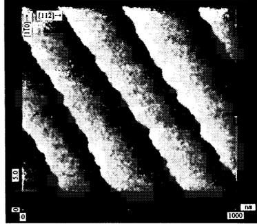
Fig.5. AFM image ( $1 \times 1 \mu\text{m}^2$ ) of Si(111) surface after  $\text{H}_2$  annealing.
