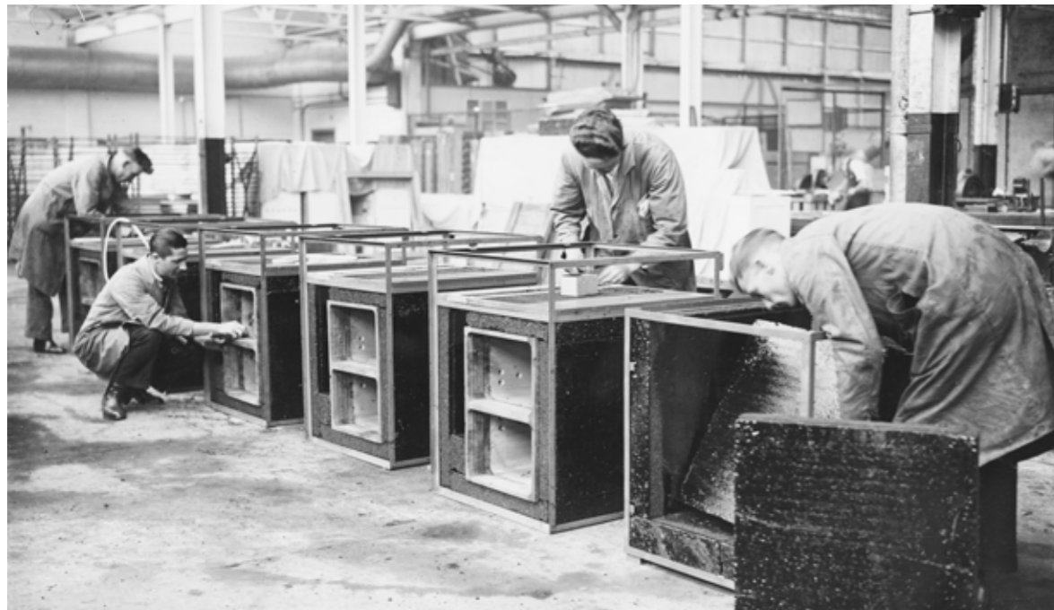
An interior from the factory in Luton where ice cream boxes with cork insulation were made – the photo is from sometime between 1927 and 1935. Absorption refrigerators were especially good for mobile icecream boxes since they could run on gas. The factory in Luton exported many such boxes to the British colonies.
