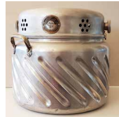
The very first Electrolux "washing machine" looked like a large, grooved cauldron and could be placed on the cooker to heat up the water. The lid was fitted with a cylinder driven by an electric motor that would rotate to press the laundry against the grooved sides of the cauldron.
