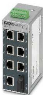
7 / 6 RJ45-Ports und 1 / 2 LWL-Ports (Multimode)
