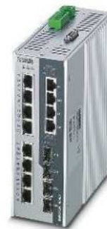
8 RJ45-PoE-Ports, 4 RJ45-Ports und 4 SFP-Ports
