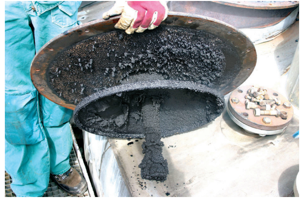
This gauge is still operating and gauging accurately despite the heavy contamination. The parabolic antenna has for several months been exposed to blown bitumen heated to 160 °C (320 °F).
