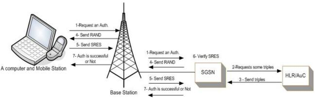
Figure 3 GPRS Authentication and ciphering
