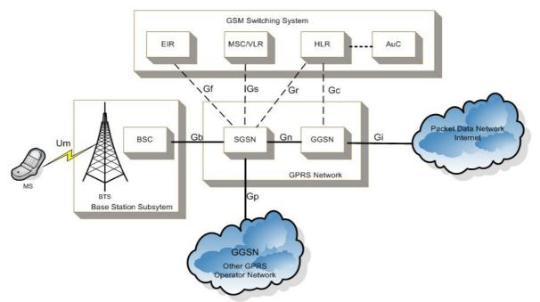
Figure 1 GPRS Architecture and Interfaces
