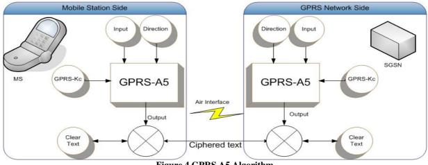
Figure 4 GPRS A5 Algorithm
