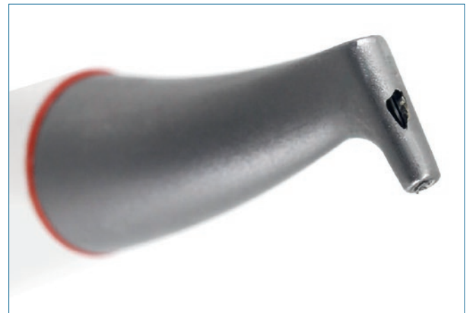
Fig. 7 The powder used must be perfectly matched to the instrument to ensure patient safety and a long service life. The image depicts the damaged nozzle of an Airflow handpiece after using a powder coated with apatite (see Fig. 5).
