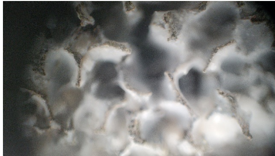
Hydrothermal conditions: 20% steam @400C/100psi 466 sccm (0.2 m/s), 24 hrs
