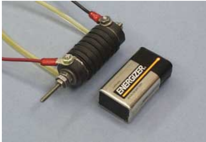
Figure 4 — A Miniature 1 W Air-Breather Alongside a 9 V Alkaline Battery.
