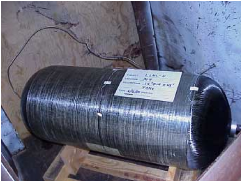
Figure 16: Tank #4 before hydroburst test
