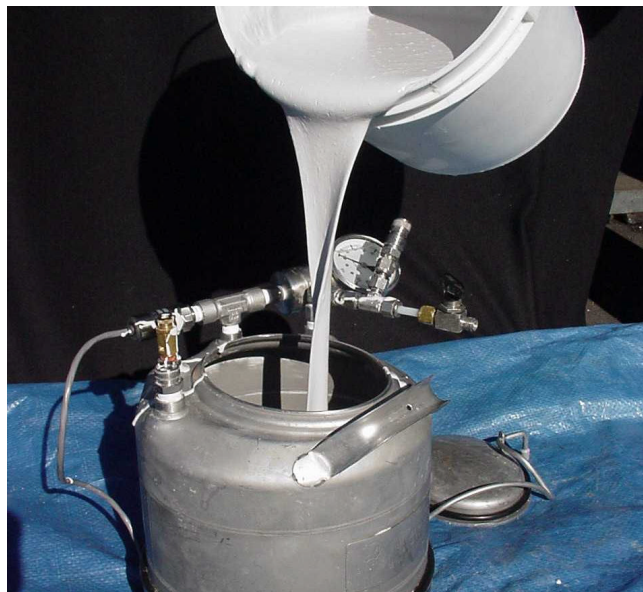
Figure 3 - Lithium Hydride Slurry
