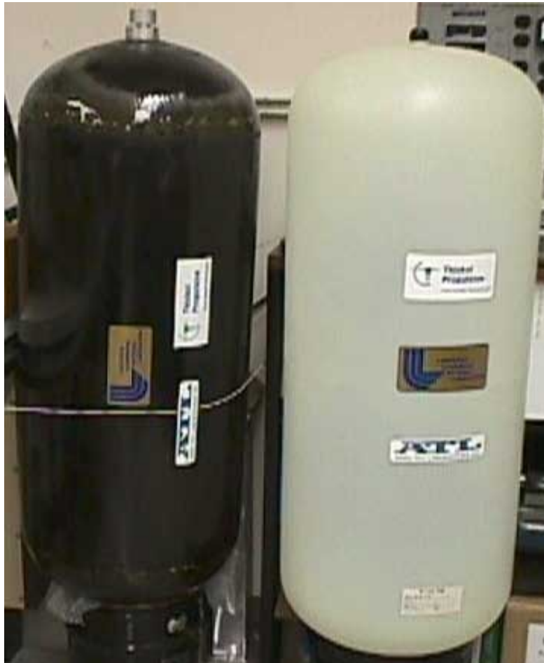
Figure 2 – First Composite Wrapped Tank Prototype Next to Thin-Wall Liner
