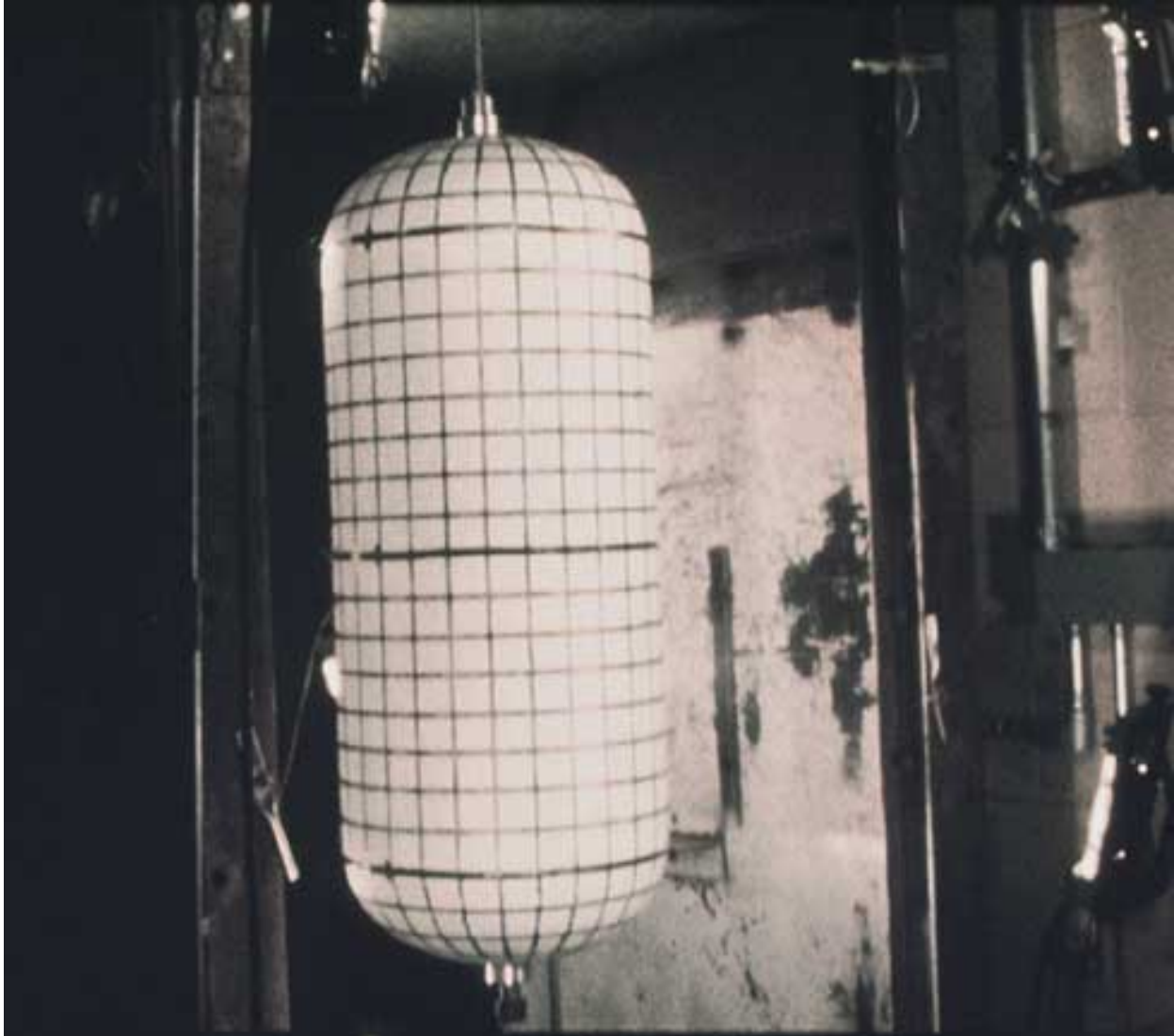
Figure 5 – Condition of Tank #5 before Highly-Instrumented Burst Test
