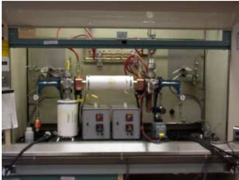
Figure 5 — Bench-scale reactor for a 100 W electrolyzer stack
