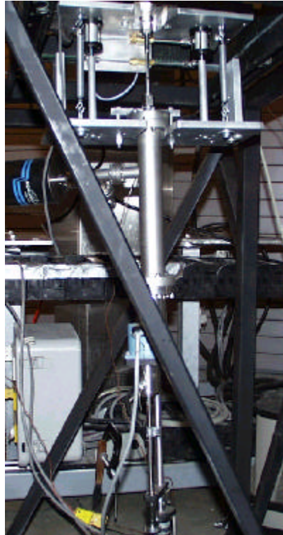
Figure 6. Particle Feeding System (below reactor assembly)
