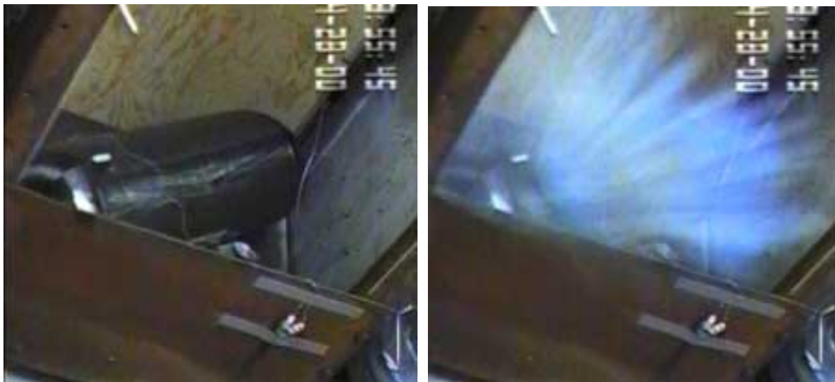
Figure 2: Tank #3 failure initiation
