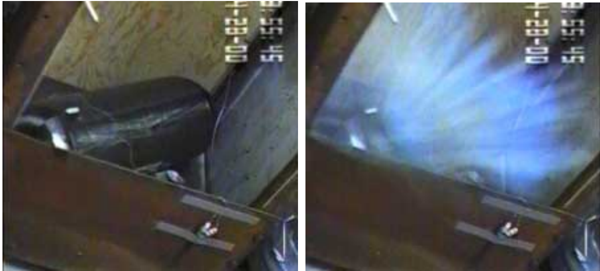
Figure 4 – Video Captures Localized Failure During Tank #3 Burst Test
