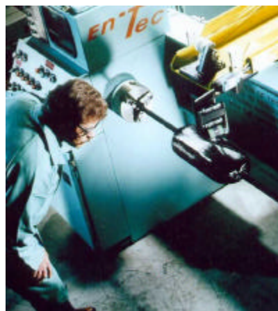
Figure 7. Filament winding a conformable cell
