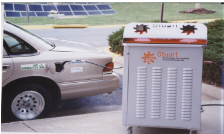
Figure 6 – P1 Model 25 Refueling NRG Hythane Vehicle at the NHA Meeting, Washington, DC
