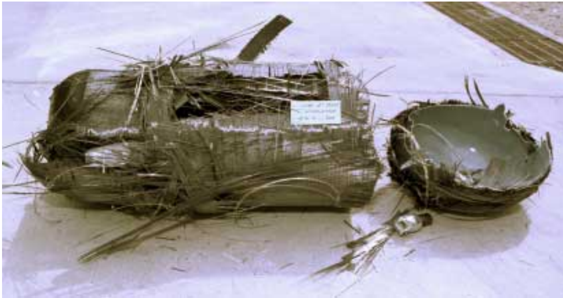
Figure 3 – Remains of Test Tank #3 after Premature Burst
