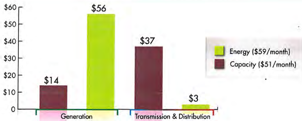
Figure 10: In Considering the Value of the Integrated Grid, Costs of Generation, Transmission, and Distribution Can Be Further Determined for Energy and Capacity.
