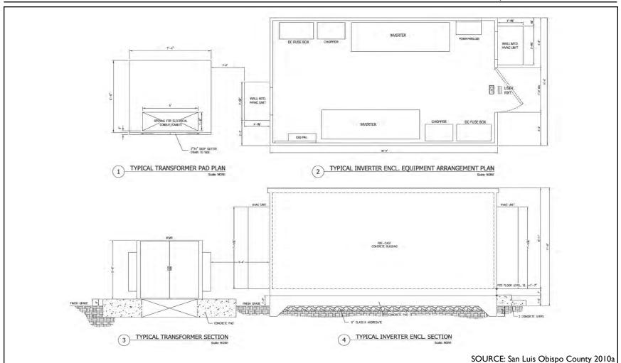
Typical PV arrays would include two inverters housed in an enclosure and one transformer. The inverters would convert the DC electric input into AC electric output, and the transformer would step up the current to 34.5 kV.
