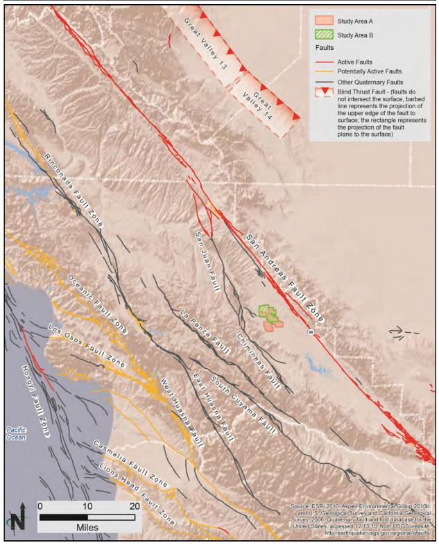
The Proposed Project is in a seismically active area. The San Andreas Fault is 2.5 miles to the east.
