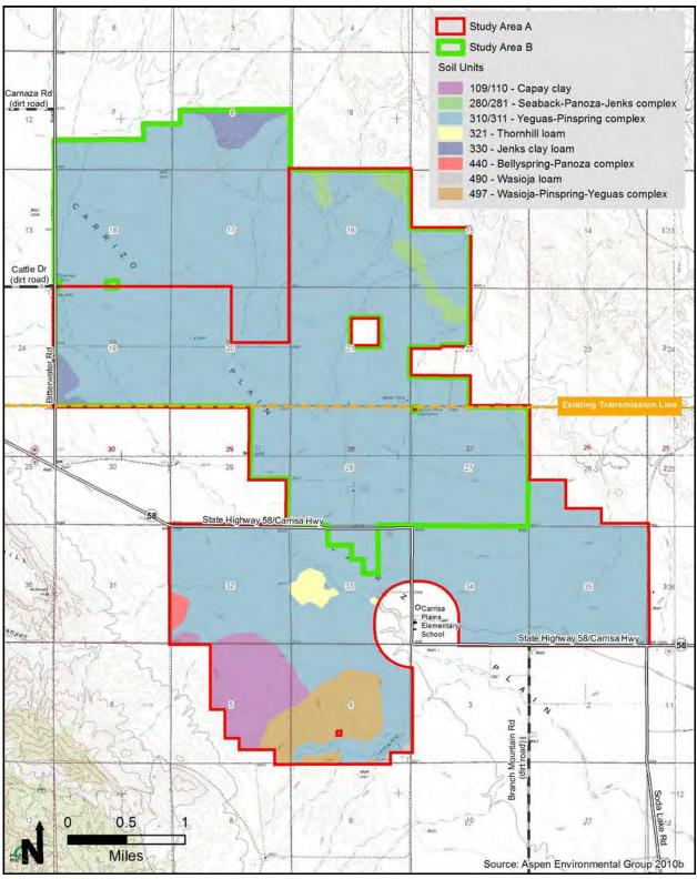
Soils in the project area are highly expansive, moderately to severely corrosive to ferrous metals, and aggressive to copper.
