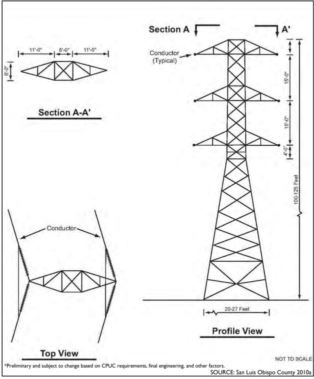
Two new 100- to 125-foot-high doublecircuit lattice steel transmission towers and four steel poles would be installed to accommodate the looping of PG&E's 230 -kV transmission line into the switching station.
