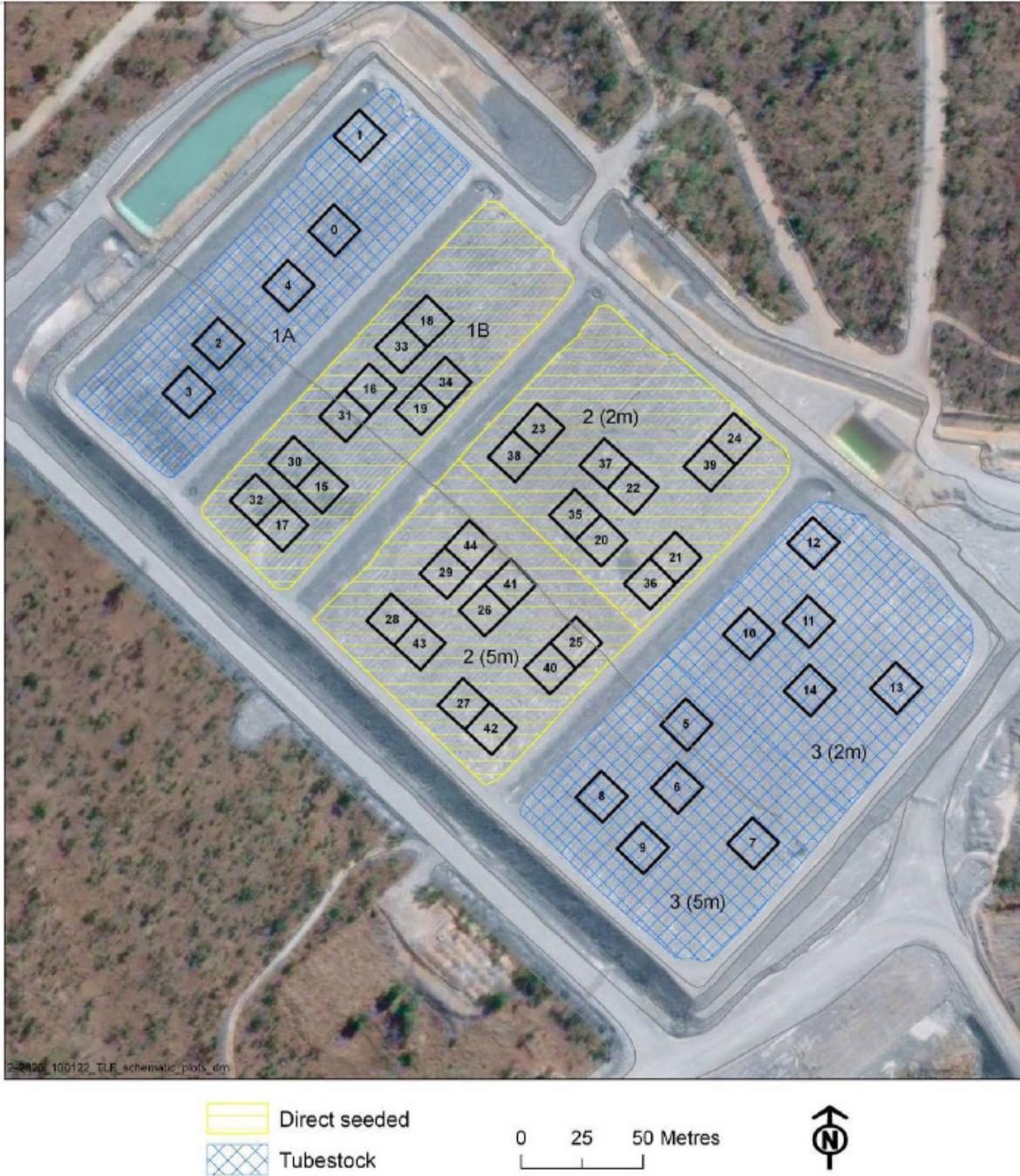
Figure 5-103: Trial Landform layout from northwest to southeast are sections 1A & 1B (waste rock only) and 2 & 3 (waste rock / laterite mix). Includes 15 x 15m permanent monitoring plot locations
