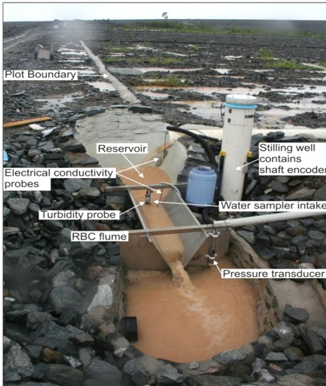
Figure 5-16: Runoff through the flume on the trial landform erosion plot 3 during a storm event (Saynor et al., 2014)
