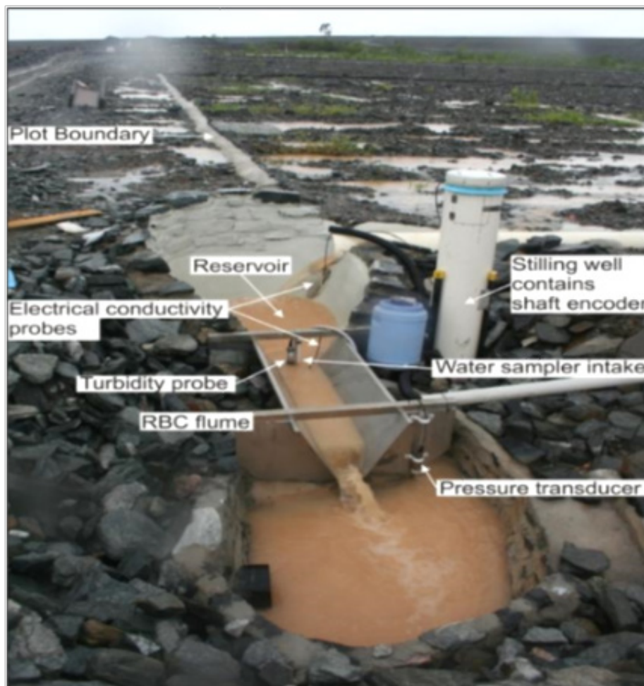
Figure 4-9: Runoff through the flume on the trial landform erosion plot 3 during a storm event (Saynor et al. , 2014)
