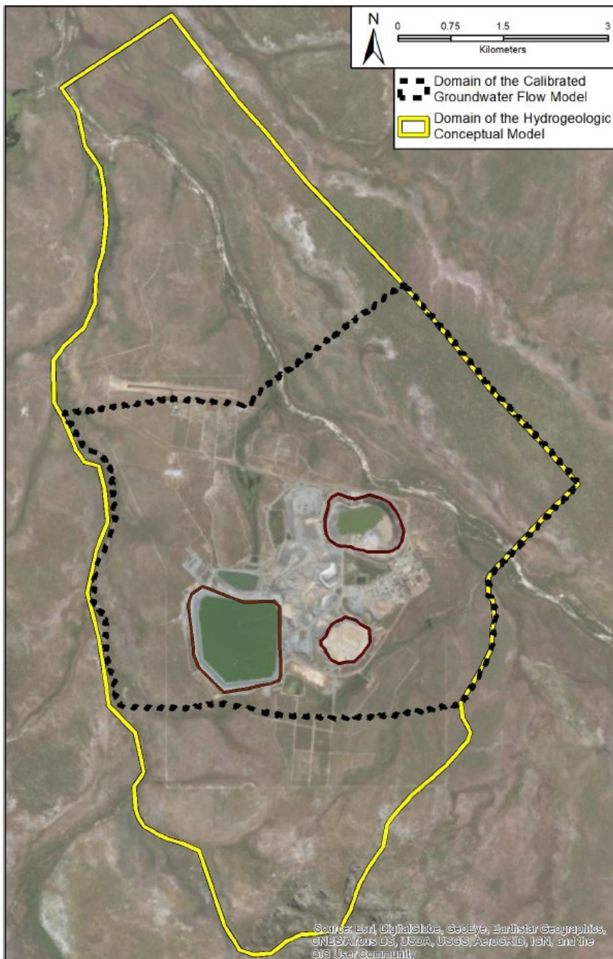
Figure 5-54 Spatial domain of the hydrogeological Ranger Mine conceptual model relative to the domain of the calibrated groundwater flow model.
