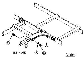
Prepare surface by sanding paint to expose bare metal
