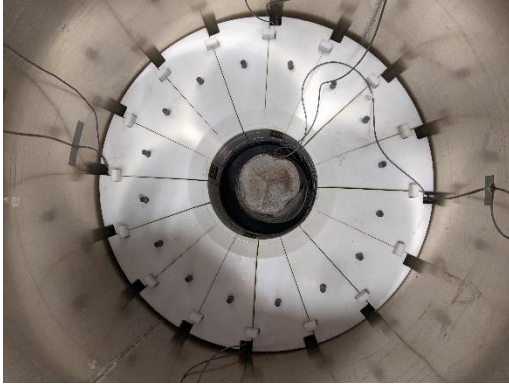
a. three layers of reflector blocks installed
