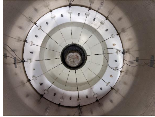
b. six layers of reflector blocks installed
