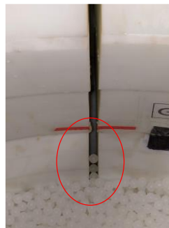
b. pebbles in gap between adjacent columns of blocks
