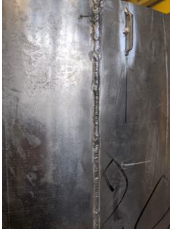
Figure 5.18. Weld on the core barrel
