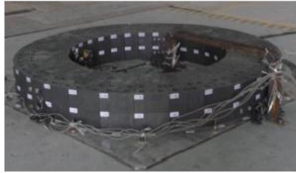
b. double-layer core model on earthquake simulator
