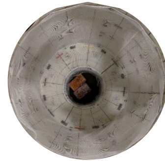
c. fabric net installed on inside the reflector-block assembly
