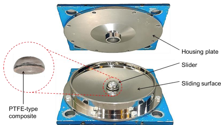
Figure A.1. Components of an SFP bearing
