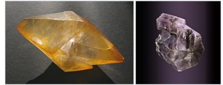
Calcite (on left) and Aragonite (on right). Both crystals are made out of calcium carbonate, making these crystals dimorphic.
