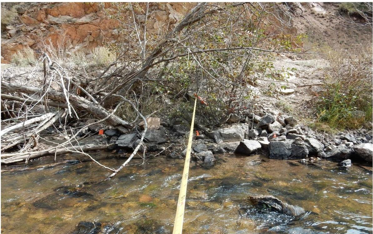
**Figure A13c. Sediment pushed into the river from road construction on the right bank.**
