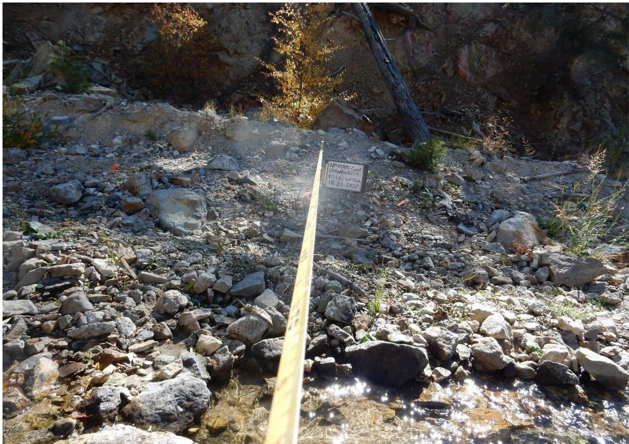
Figure A13g. Splays of sediment have buried the channel with new cobble/gravel bars and sheets.
