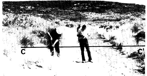
Figure 5. Reference points for bankfull level (C-C') in a reach of an ephemeral-stream channel in New Mexico.
