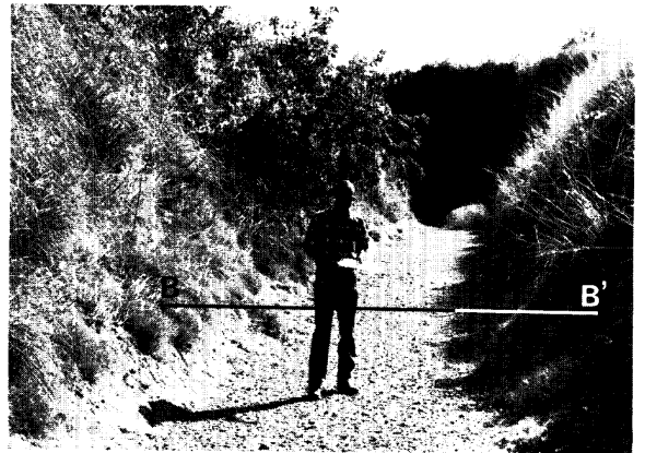
Figure 6. An incised channel in southeastern New Mexico with well-defined active-channel reference points (B-B') but lacking a defined bankfull level.
