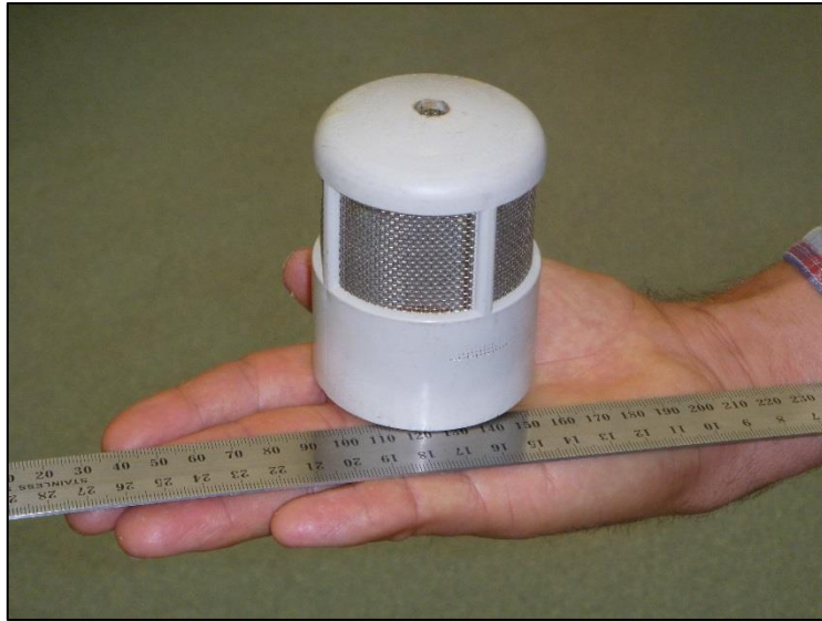
Figure 6. Air vent cowl used to hold bait.
