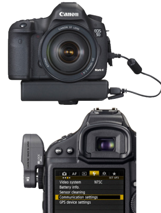
▲ Some WFTs are quite bulky and fit to the base of the camera (top WFT-E7). Others are smaller and attach to the side of the camera (above WFT-E6).
