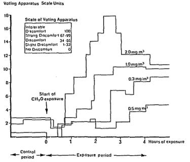
Figure 7 Variation with time of the mean discomfort vote in scale units at four different concentrations of formaldehyde In the control period, clean air was supplied to the subjects.
