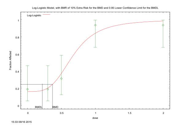
Figure 8a. BMDS Version 2.2 Fitted Log-Logistic Dose-Response Model for Sensory Irritation Using the Data at the 4 Positive Doses and Assuming 3 Responses at Dose 0. Copied from Figure B4 of the IRIS Report (EPA, 2022).
