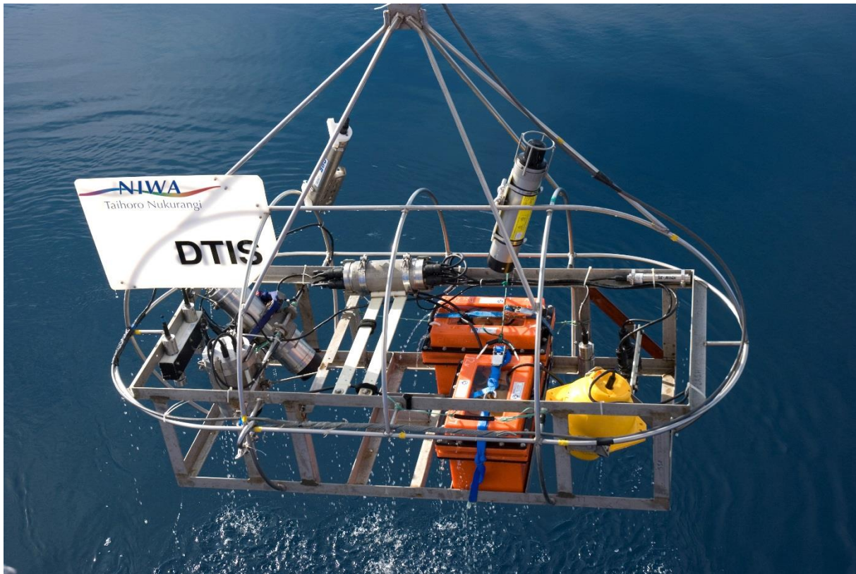
Figure 2-7: NIWA's Deep Towed Imaging System used to take images of the seafloor during OS20/20 surveys. [photo: NIWA]
