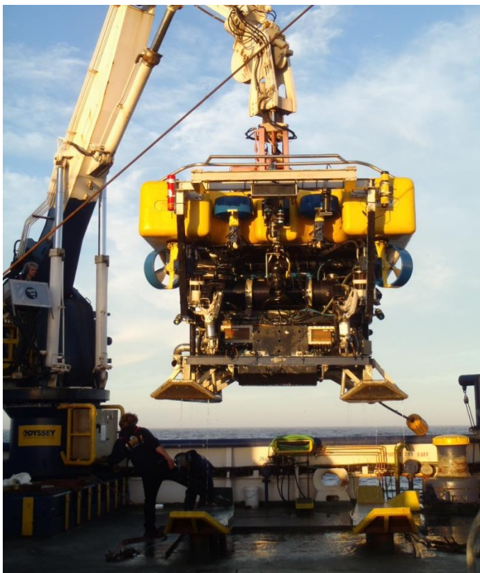
Figure 2-6: Remotely operated vehicle (ROV) Zeus II used to take images of the seafloor and obtain multi-beam echo sounder data. [photo: Emily Jones, Golder Associates].
