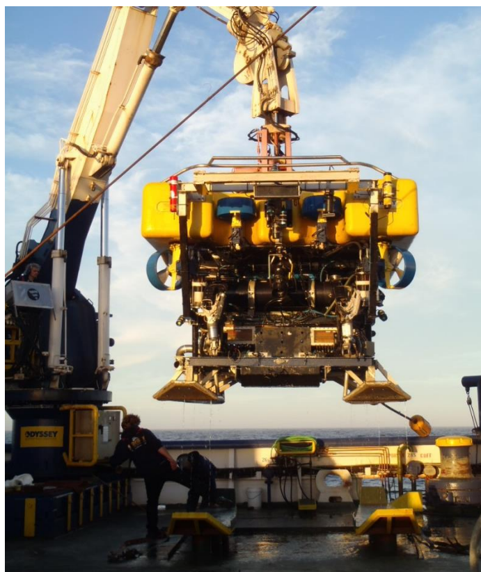
Figure 2-3: Remotely operated vehicle (ROV) Zeus II used to take images of the seafloor and obtain multi-beam echo sounder data. [photo: Emily Jones, Golder Associates].
