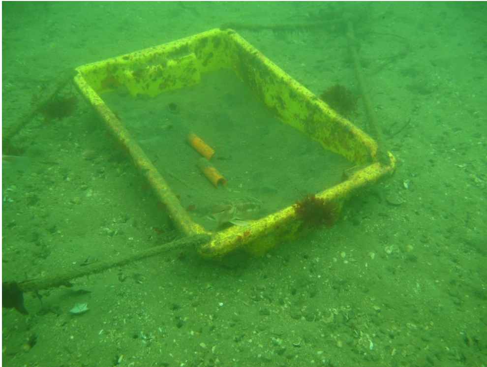
Figure 81: Experimental treatment at Mahanga Bay, taken 1/8/2012. Note that some of the experimental sand has been scoured out of the fish-bin.
