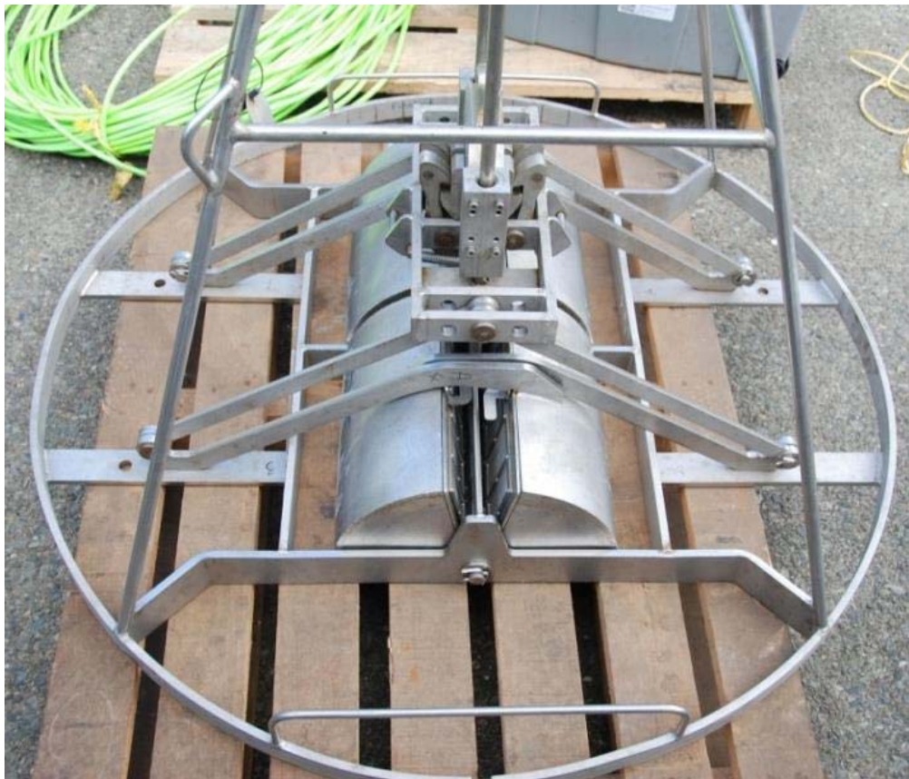
Figure 5 The double Van-Veen grab sampler used for benthic sampling
