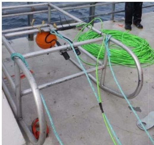
Figure 6 The video sled used for collecting seafloor footage in 2016
