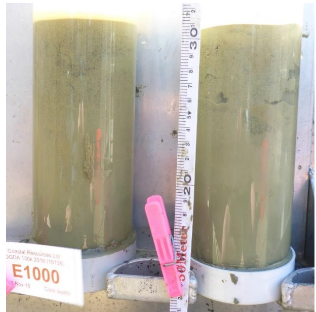
Figure 8.15 Sediment Gravity Cores – E 1000, 23 November 2016
