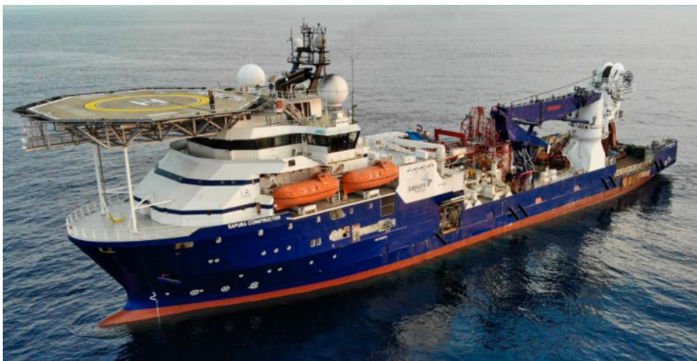
Figure 6 Example of a WIV – the Sapura Constructor
