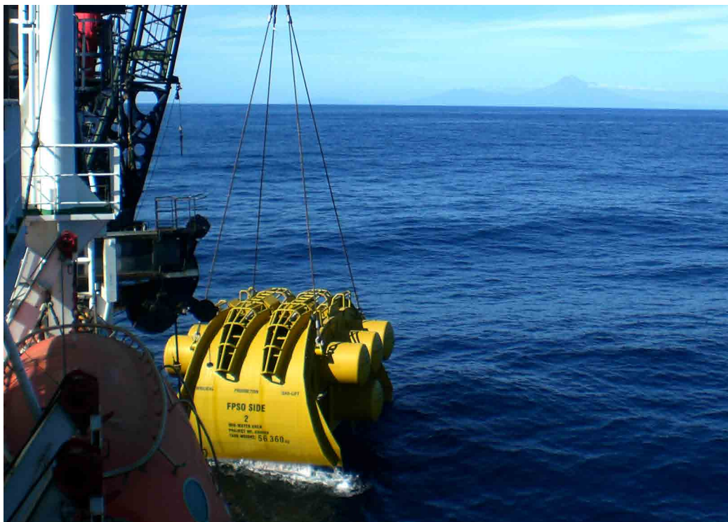
Figure 8: A Mid Water Arch being lowered into position at Tui in 2007
