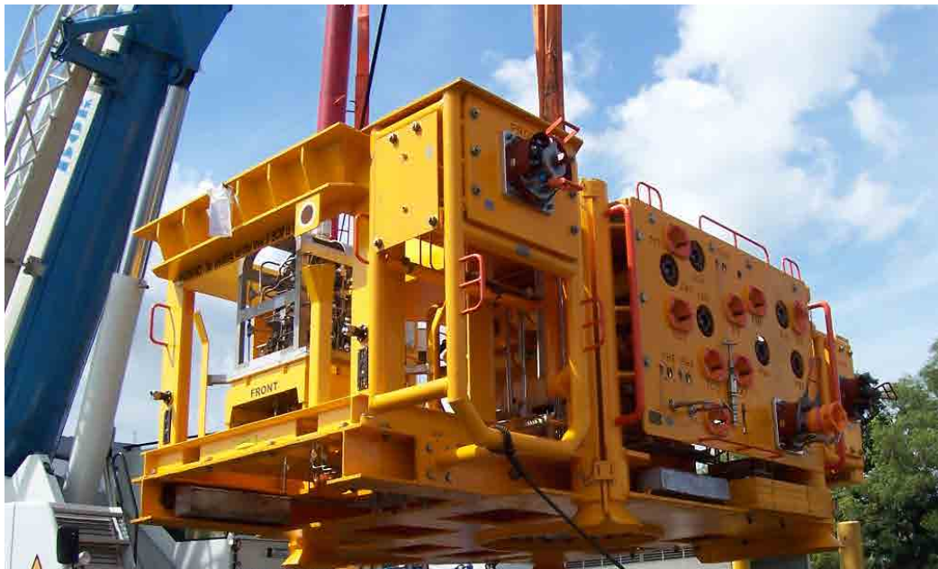
Figure 9: A Subsea Xmas Tree prior to installation in the field in 2007
