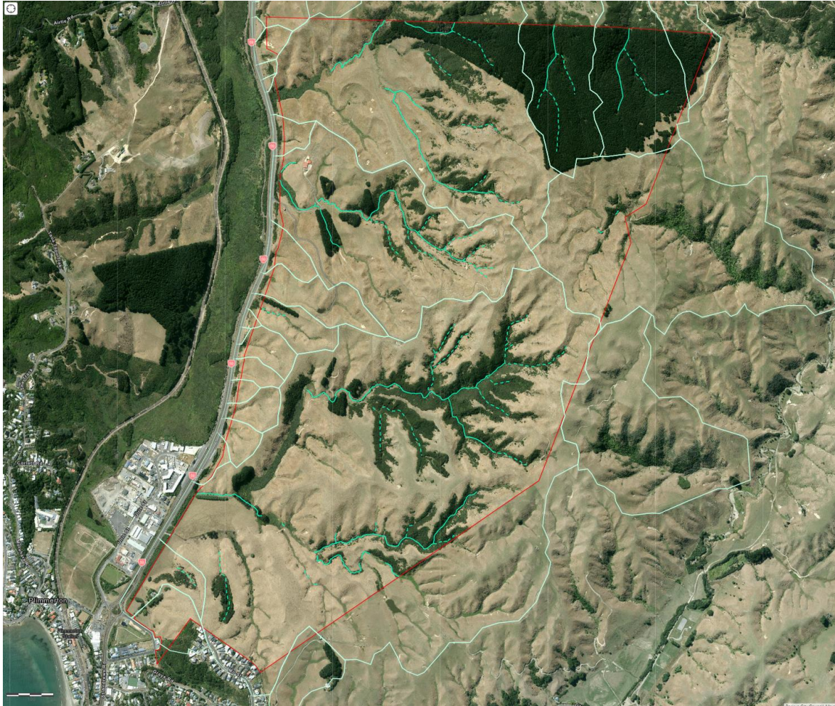
Figure 9. Site catchments and sub catchments. Streams (solid and dashed turquoise lines), catchments (white lines), site boundary (red line).
