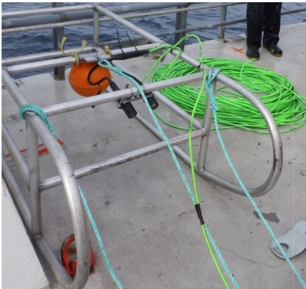
Figure 5 The Video Sled used for Collecting Video Imagery of the Seabed Environment
