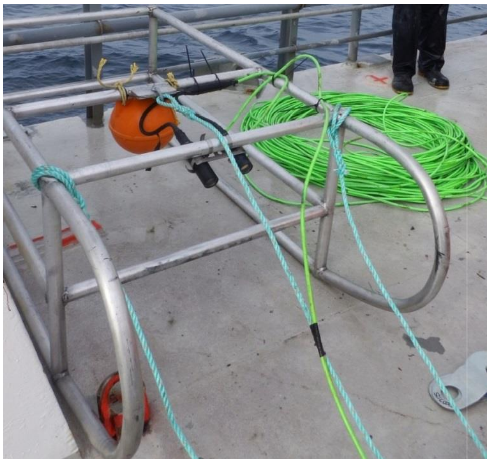
Figure 5 The Video Sled used for Collecting Video Footage of the Seabed Environment
