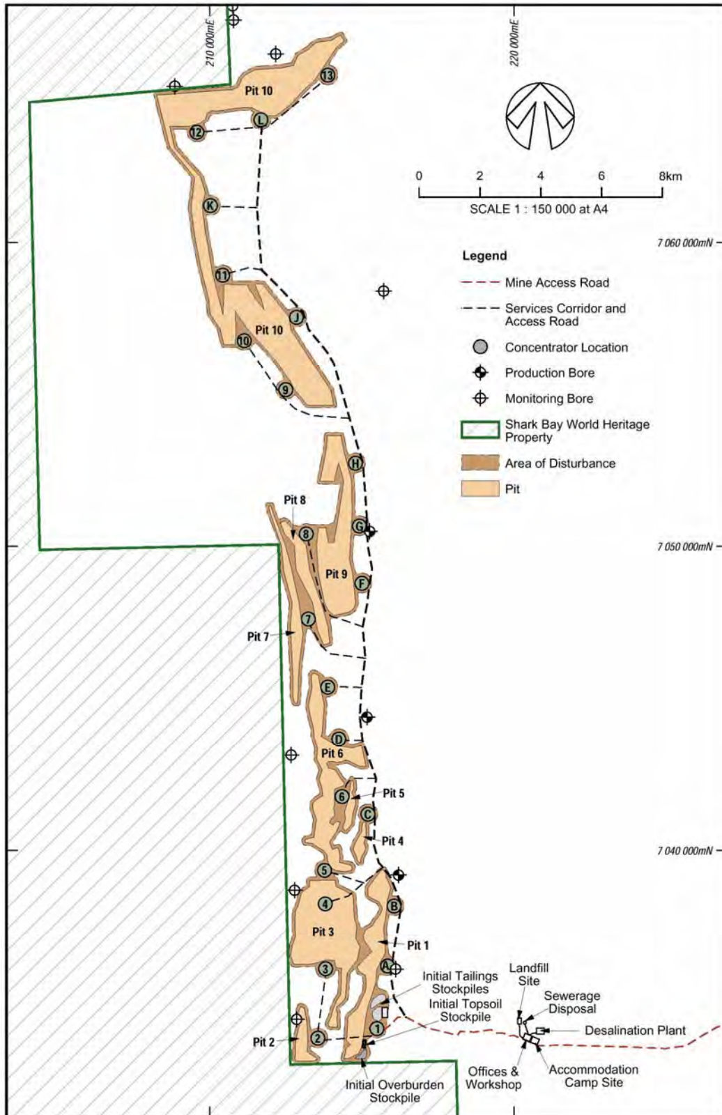
Figure 2.1: Proposed Layout of Amy Zone Operations of the Coburn Mineral Sand Project
