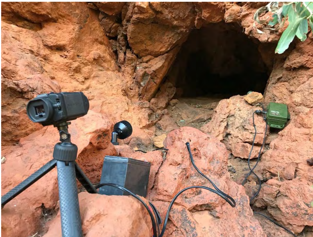
Plate 1 Video camera, IR lamp and detector set at South Star Pool cave complex
