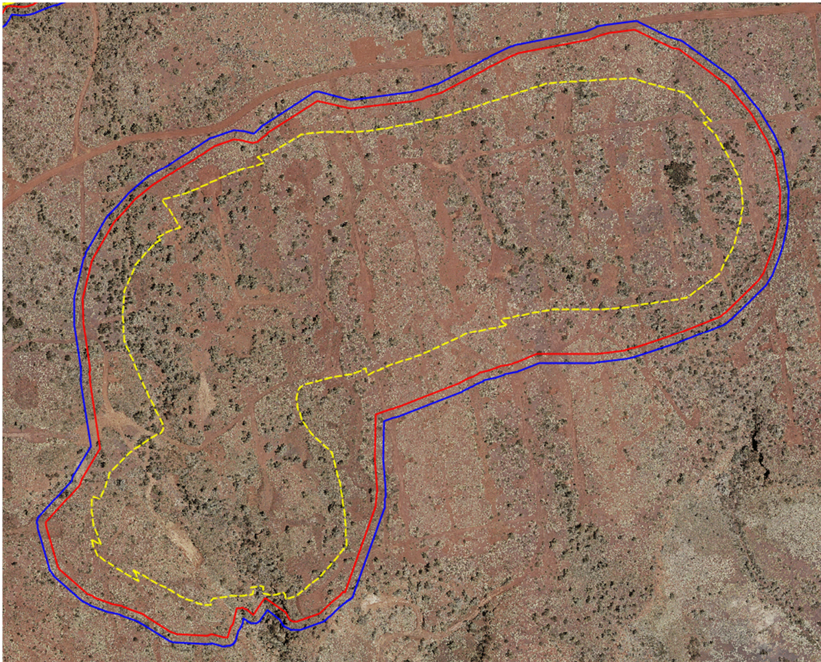
Figure 33: Example of abandonment bund placement (blue), outside the ZOI (red) and the pit crest (yellow)
