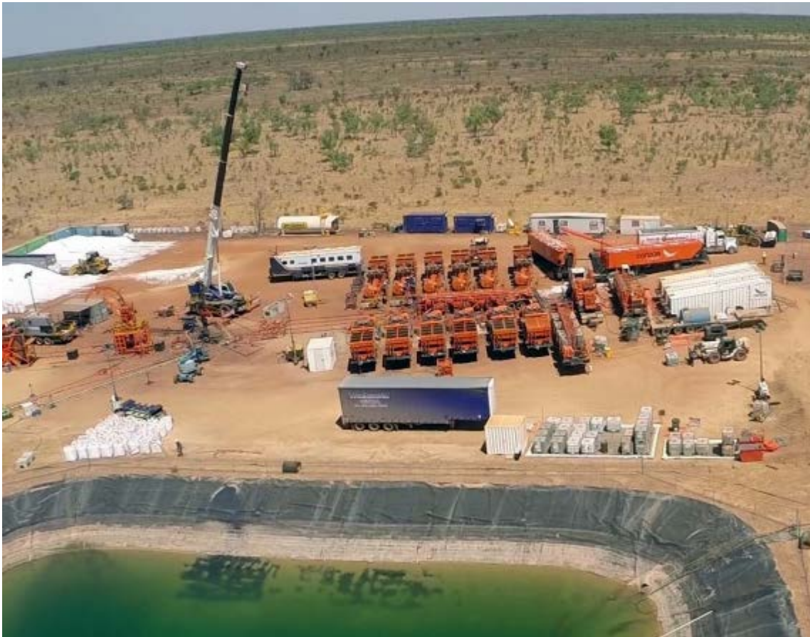
Figure 2-2: Typical HFS layout
