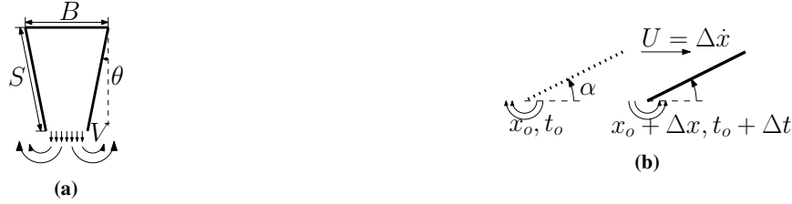
Figure 1: a) Schematic of the vortex generator designed by Leweke and Williamson [1] b) Schematic of the starting/stopping vortex pair generator used in the present study
