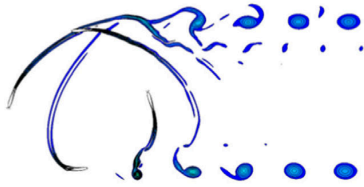
Figure 3: Simulated operation of a Darrieus turbine with a dual (+10°/-5°) circulation constraint [7].
