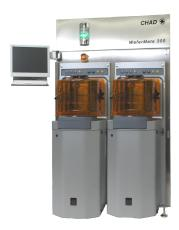
As a class-1 clean FEOL (front-end-of-the-line) EFEM, the *WaferMate300*™ includes all applicable mini-environment components, E84 compliance, and rear hand-off.
