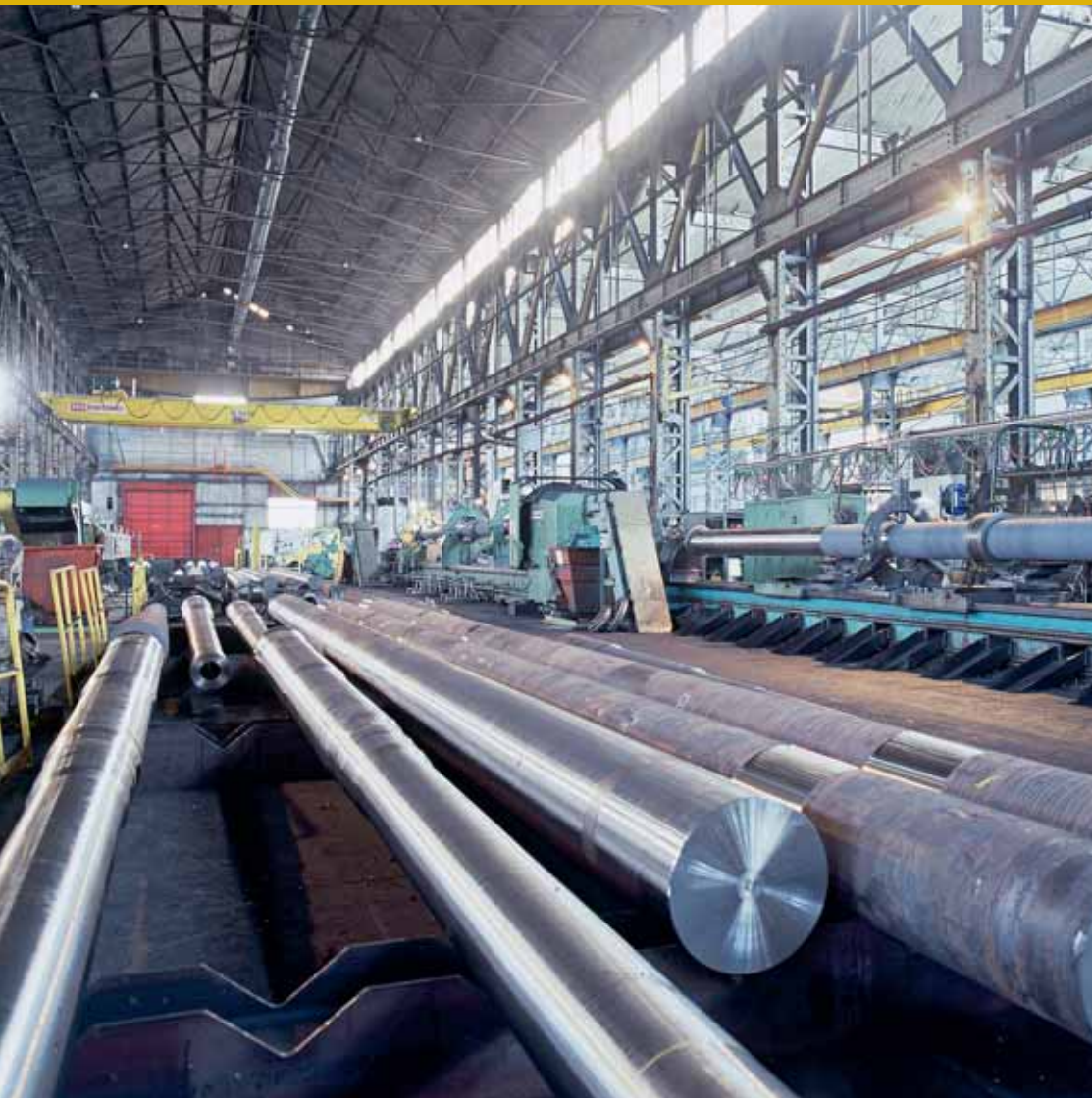
AUBERT & DUVAL'S FIRMINY (FRANCE) PLANT SPECIALISES IN MANUFACTURING LONG CLOSED DIE-FORGED PARTS.
