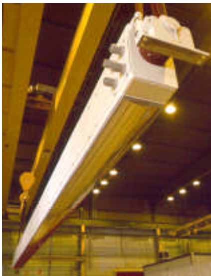
IQTension is an unique on-line system for measuring web tension contactless and continuously across the entire width.
