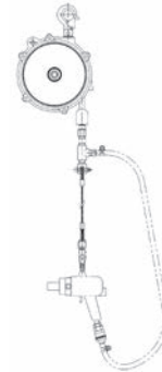
ATB-1 fitted with horizontal tool hanger
