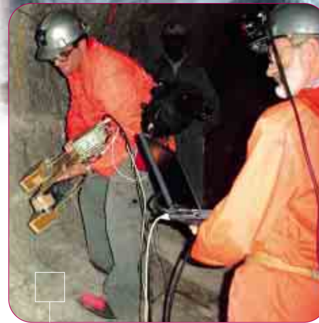
The CRIS device helps to detect cracks in mine walls
