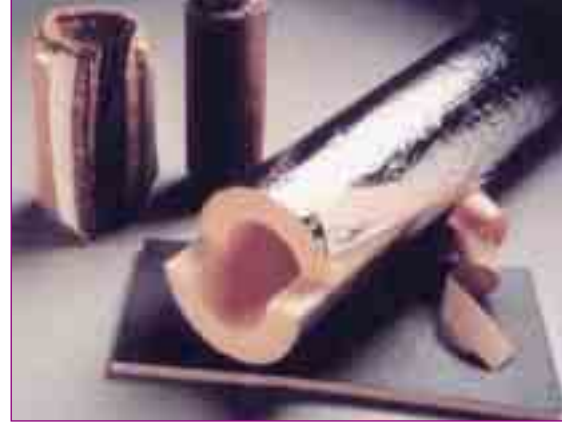
Foam insulation and metalised polymer blankets developed for space are now being used in terrestrial applications
