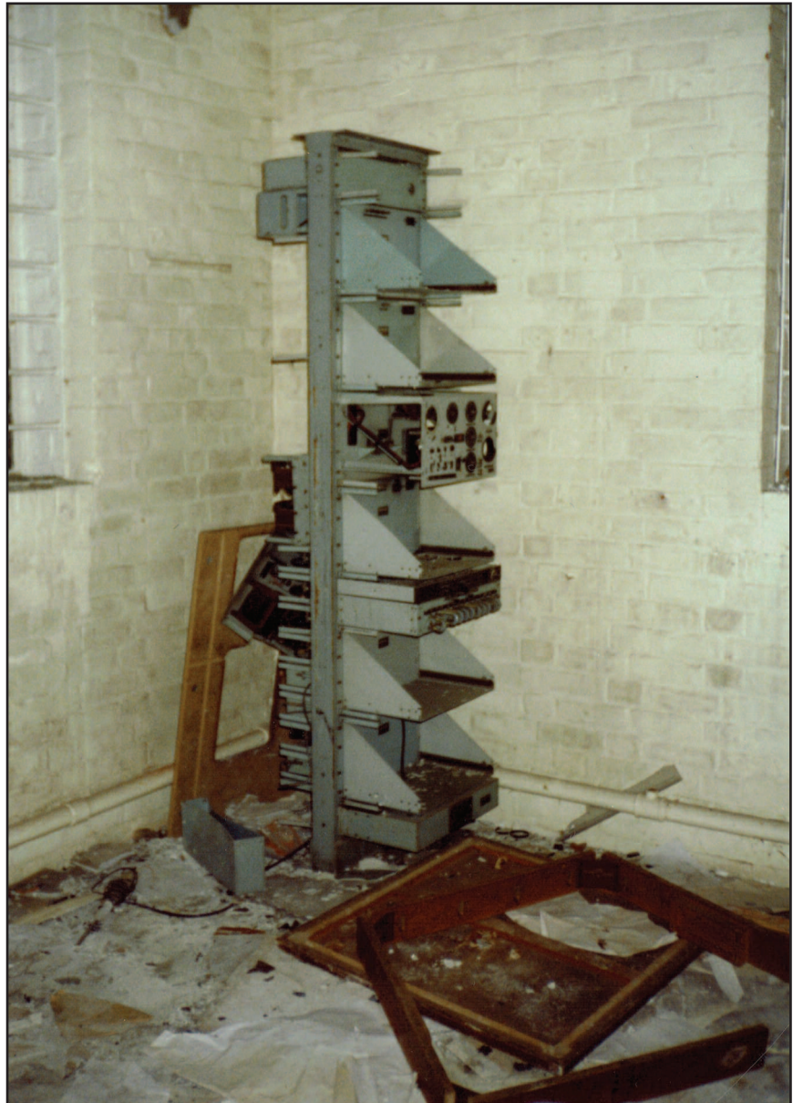
8. The remains of one of the Mullard PO-W22 R/T receivers. It had been removed from its original position in the West Wing and was found by the author in a room in the derelict station buildings when he visited the site. (Author photograph, July 1996)
