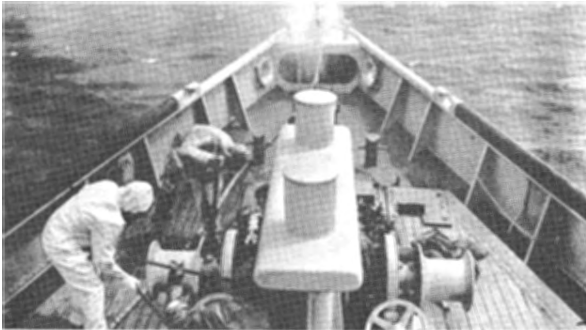
Figure 37. Shipboard decontamination using high-pressure seawater and scrub brushes, CASTLE.
