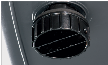
Drainage plug open
