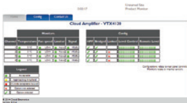
WM-1 web interface homepage showing a summary of the information from each unit available to the site host.
