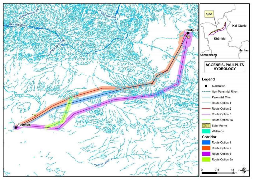
Figure 4: Hydrology of the area that the proposed 400kV powerlines corridor alternatives are situated in (as per the existing NFEPA spatial layers)
