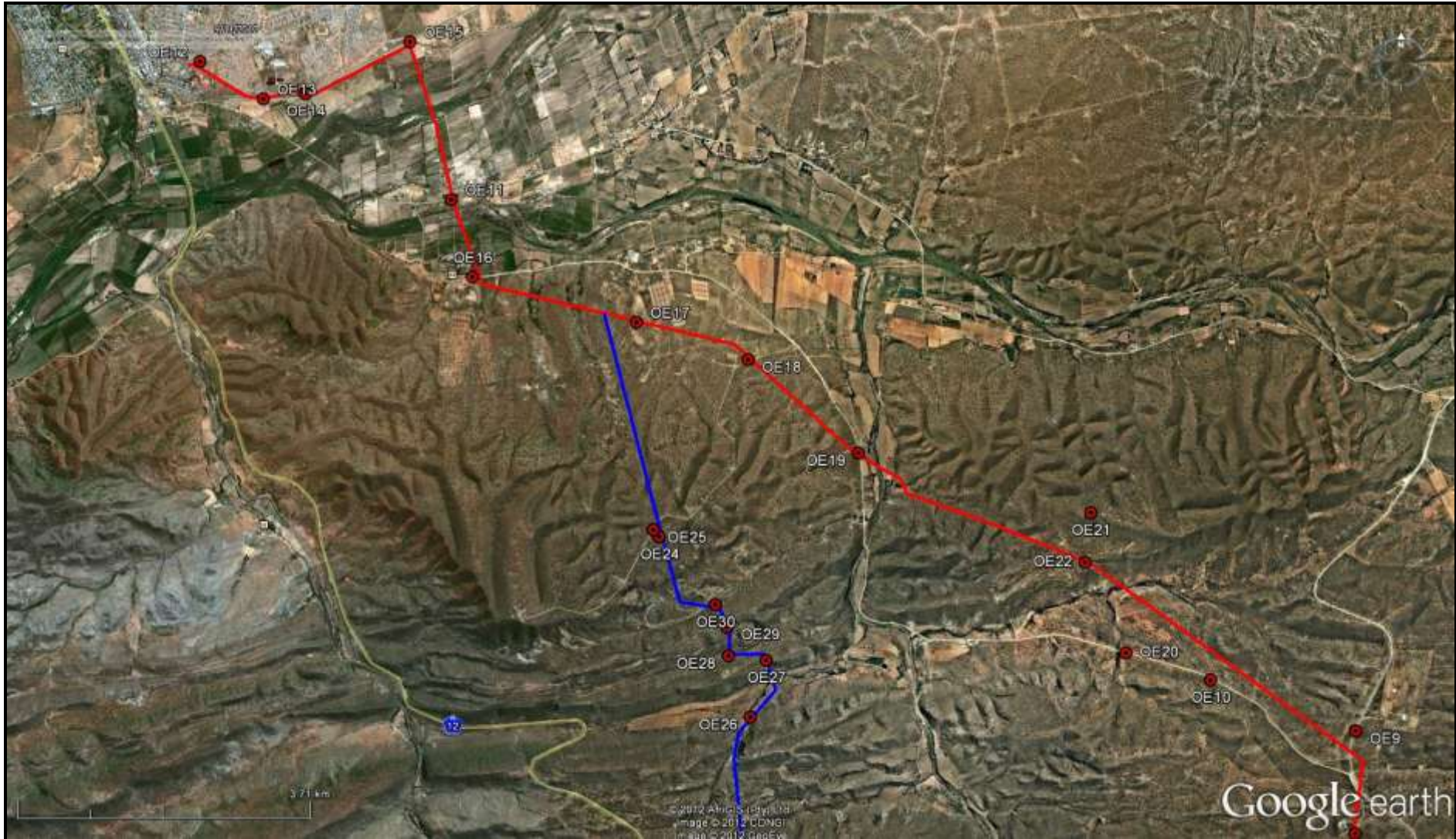
Figure 28. Aerial image (Google Earth™) of the northern part of the study area showing the convergence of the two proposed alternative transmission line routes Alternative 1 – red; Alternative 2- blue), with sample waypoints shown as OE#.
