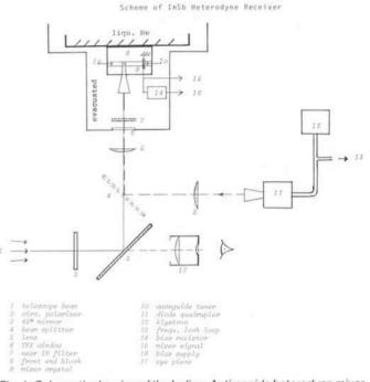
Fig. 1: Schematic drawing of the Indium Antimonide heterodyne mixer receiver (0.65 mm wavelength). The crystal sits within a front-end block with a horn antenna and a tunable waveguide circuit; its dimensions are  $0.04 \times 0.04 \times 0.2$  mm. The local oscillator is a microwave klystron plus a Schottky diode quadrupler. Matching of the telescope beam to the beam shape of the horn antenna is done with lenses. The 45° mirror can be quickly exchanged by an eyepiece for optical pointing.
