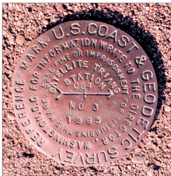
Figure 1.15 Horizontal control point marker cemented in the ground. Courtesy of the National Oceanic and Atmospheric Administration.
