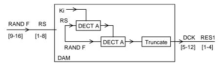
Figure G.2: Functionality of a DAM for PP authentication
