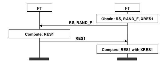
Figure 4.1: Authentication of PT (type 1 procedure)
