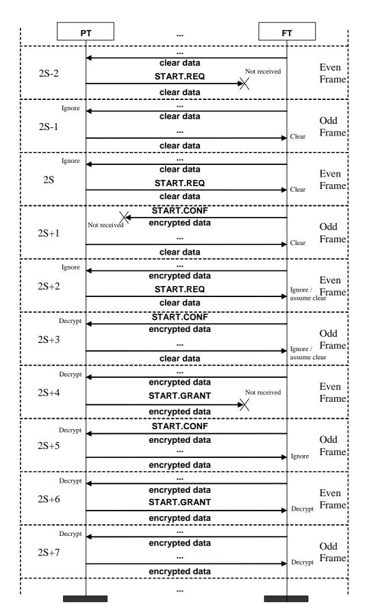
Figure 6.9: Encryption start - poor link example
