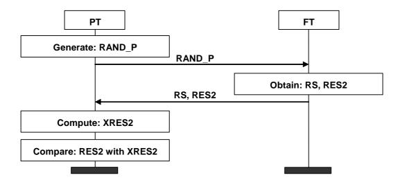
Figure 4.2: Authentication of FT (type 1 procedure)
