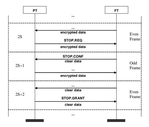
Figure 6.10: Encryption stop - good link example
