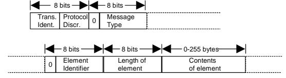
Figure 6.1: NWK Layer Message Structure (NLMS)
