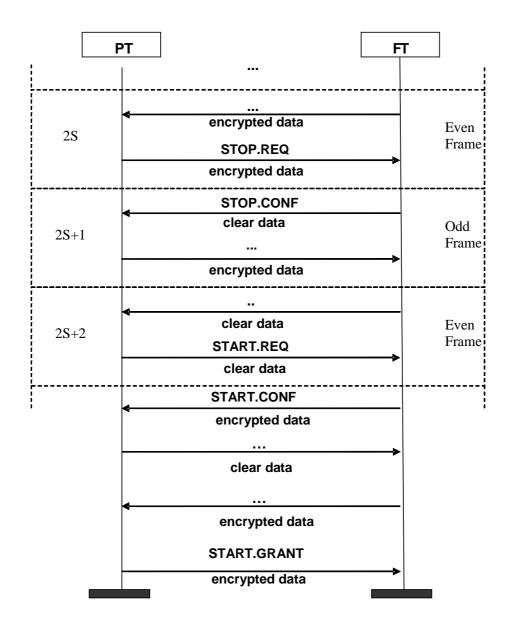
Figure 6.11: Encryption change - good link example
