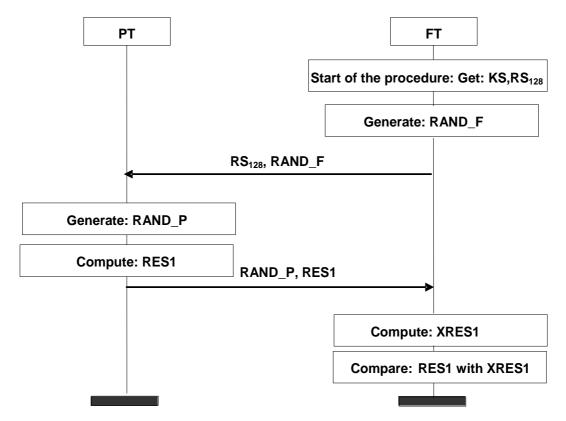
Figure 4.3: Authentication of PT (type 2 procedure)
