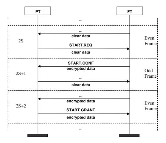
Figure 6.6: Encryption start - good link example
