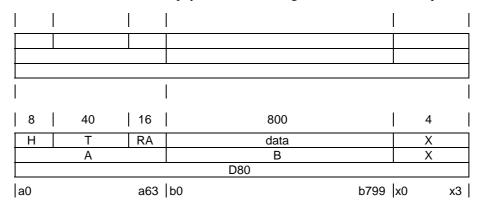
Figure 6.15: Double slot field structures
