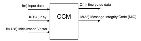
Figure 4.12: CCM Authenticated Encryption
