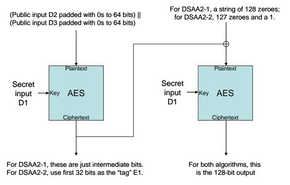
Figure L.1: The DSAA2-1 and DSAA2-2 algorithms
