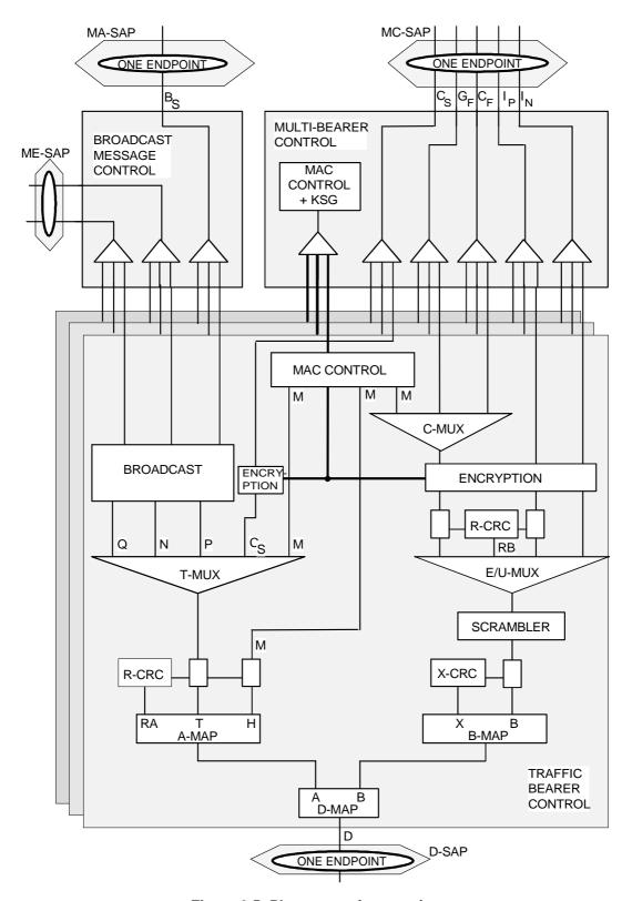
Figure 6.5: Placement of encryption
