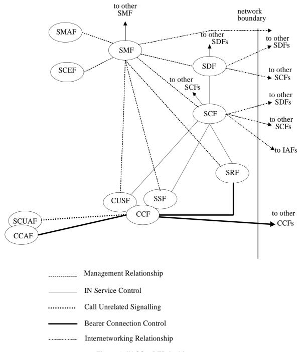
Figure 1: IN CS-3 DFP Architecture
