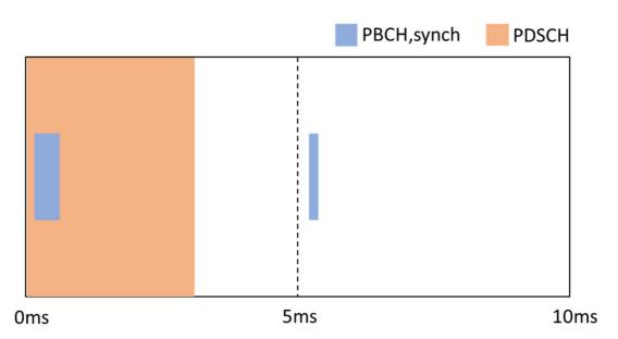
Figure J.2: PDSCH load is concentrated in time, but uses the full bandwidth
