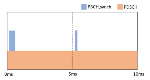
Figure J.1: PDSCH load is equally distributed in time (used bandwidth is constant)
