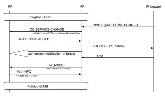
Figure D.10: Service Change from Wideband to Narrowband; re-negotiation initiated from IP-Network
