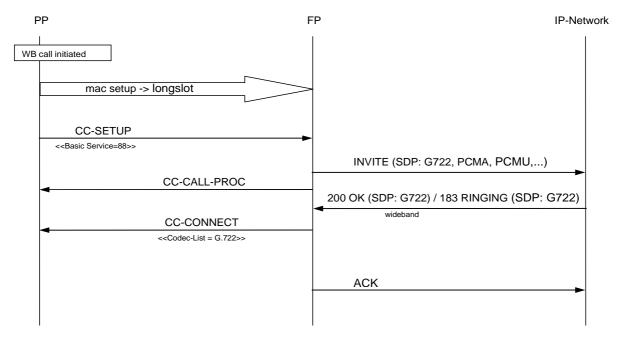
Figure D.1: Outgoing wideband call, no codec list, ITU-T Recommendation G.722 [17] chosen
