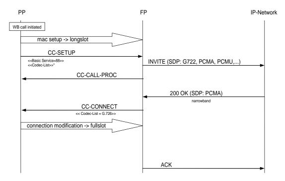
Figure D.5: Outgoing Call Wideband, negotiation results in Narrowband
