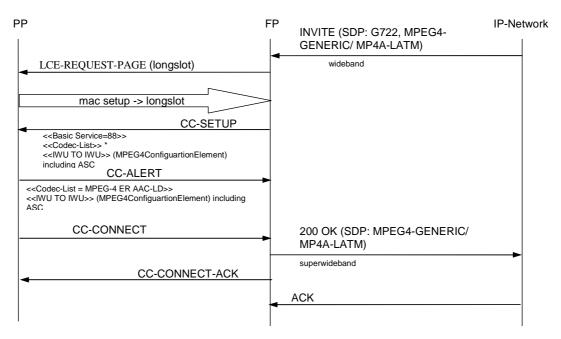
Figure D.46: Incoming Call Super-wideband, codec MPEG-4 ER AAC-LD
