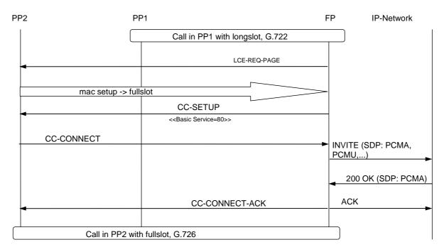
Figure D.19: Internal Call transfer from a NG PP to a PP which does not support wideband
