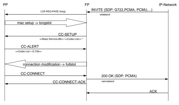
Figure D.8: Incoming Call Wideband, negotiation results in Narrowband
