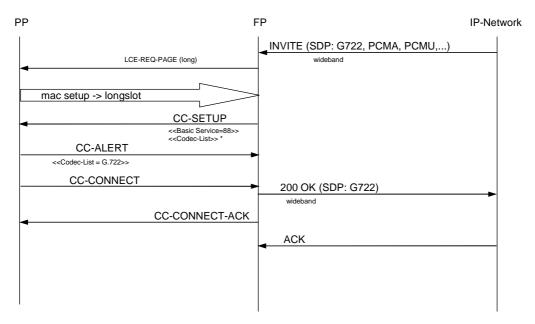
Figure D.7: Incoming Call Wideband, negotiation results in Wideband
