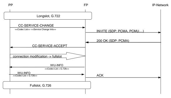
Figure D.12: Service Change from Wideband to Narrowband; PP initiated; IP Network accepts Narrowband Codec
