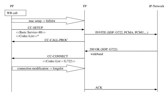
Figure D.6: Outgoing Call Wideband, negotiation results in longslot
