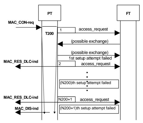
Figure 9: Bearer setup attempt fails N200+1 times
