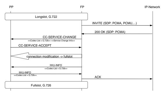
Figure D.11: Service Change from Wideband to Narrowband; re-negotiation initiated from FP
