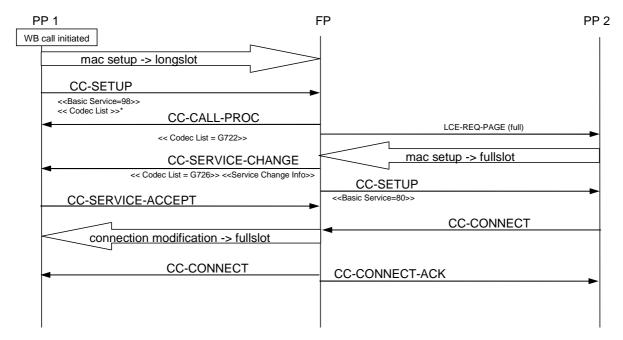
Figure D.17: Intercom Call with Interworking: WB Handset -> NB Handset, alternative procedure
