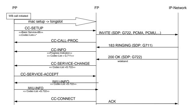
Figure D.4: Outgoing call with progress indicator; with negotiation results in CC-INFO codec change in 200 OK
