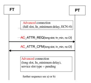
Figure D.29: Successful FT initiated connection modification (full slot  $\ln I_N$ \_minimum\_delay ->  $\log \operatorname{slot} I_N$ \_minimum\_delay), initial connection is an advanced connection
