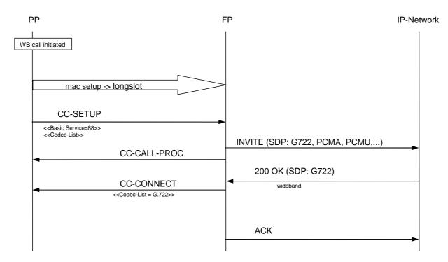
Figure D.2: Outgoing Call Wideband, codec list, negotiation results in Wideband
