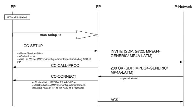
Figure D.45: Outgoing Call Super-wideband, codec MPEG-4 ER AAC-LD
