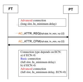
Figure D.33: FT initiated connection modification (long slot I<sub>N</sub>\_minimum\_delay -> full slot I<sub>N</sub>\_minimum delay)
