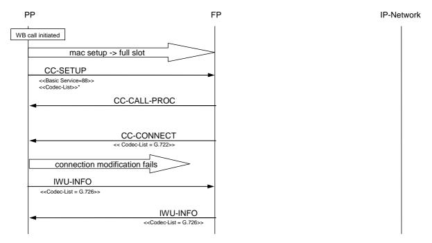
Figure D.26: Outgoing Call, slot type modification fails
