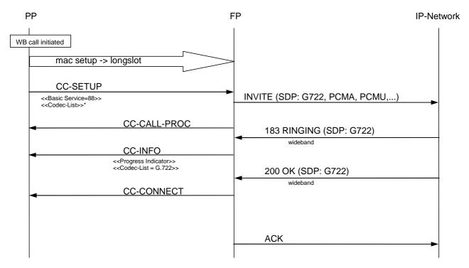
Figure D.3: Outgoing call with progress indicator with negotiation results in CC-INFO
