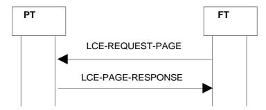
Figure 5: Indirect FT initiated link establishment
