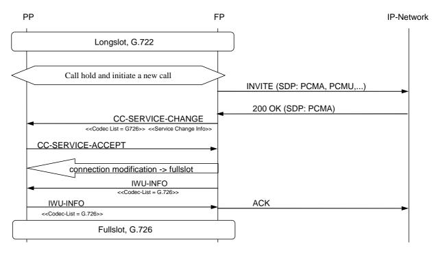
Figure D.23: Service Change from Wideband to Narrowband with Call Hold
