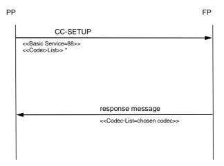
Figure 4: Codec Negotiation during call setup
